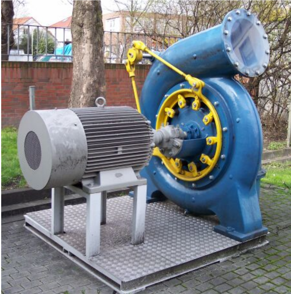
Figure 2-28: A Francis turbine connected to a generator. [61] Licensed under CC BY-SA 3.0
