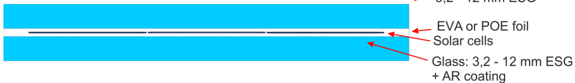
Figure 3-23: Glass-foil vs glass-glass solar module. [94]
