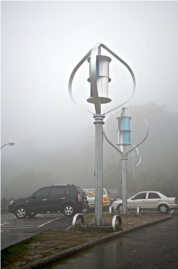
Figure 1-31: Combination turbines of Darrieus and Savonius designs in Jinguashi, Taiwan. [30] Licensed under CC BY-SA 3.0
